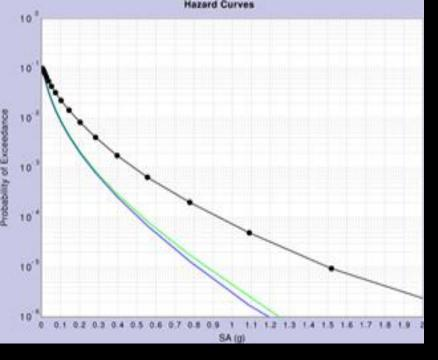
Probabilistic Seismic Hazard Analysis (PSHA) curve. Estimates the probability that earthquake ground motions will exceed some intensity measure.
