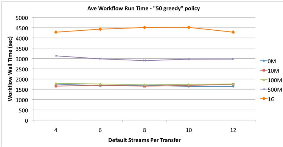
Fig. 5. Shows the effect on workflow execution time of increasing the file size of the additional staged data for 50 stream threshold and increasing number of default streams per transfer.
