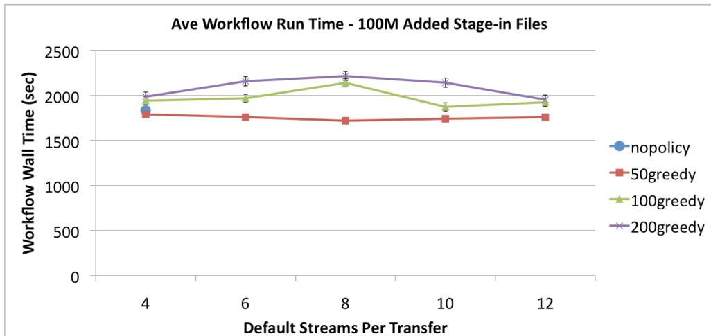
Fig. 7. Workflow Performance with staging of additional 100 MByte files.
