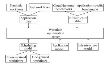
FIGURE 1: An overview of our approach to workflow scheduling. Mathematical models are input to the solver: application, infrastructure, and scheduling models, together with corresponding datasets.
