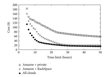
FIGURE 8: Optimal cost found by the coarse-grained scheduler for Montage workflow of 500 tasks with runtimes artificially multiplied by 1000 for different cloud infrastructures.
