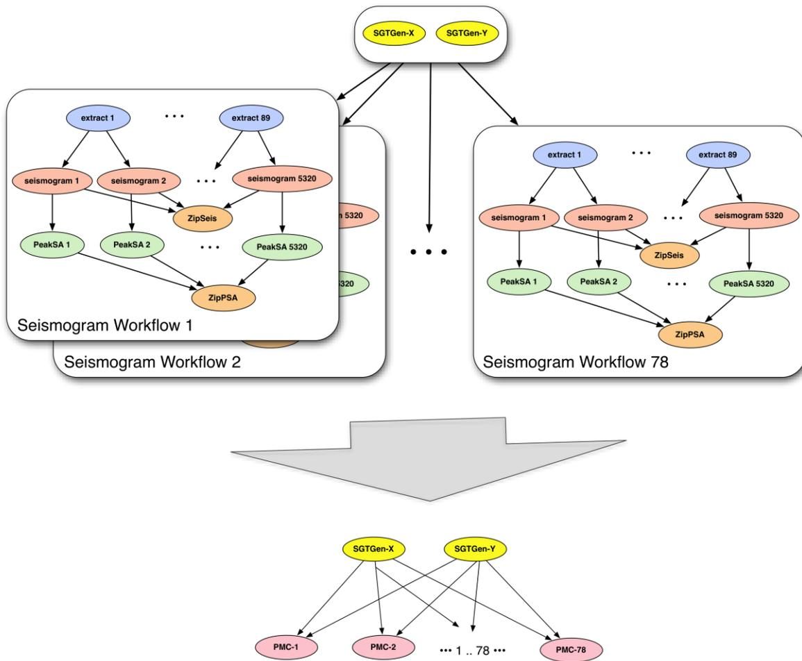
**Figure 6. The CyberShake hierarchical workflow containing two wave propagation simulations (SGTGen-X, SGTGen-Y) and 78 seismogram workflows. The figure shows the workflows being mapped to 80 pegasus-mpi-cluster jobs for execution on NICS Kraken**
