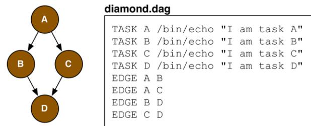
Figure 2. Example diamond-shaped workflow (left) and corresponding pegasus-mpi-cluster DAG file (right).
